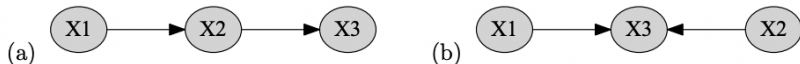
Figure 3.2.3: Directed graphs representing (a) X_1 \perp\!\!\!\perp X_3 \mid X_2 and (b) X_1 \perp\!\!\!\perp X_2 .
